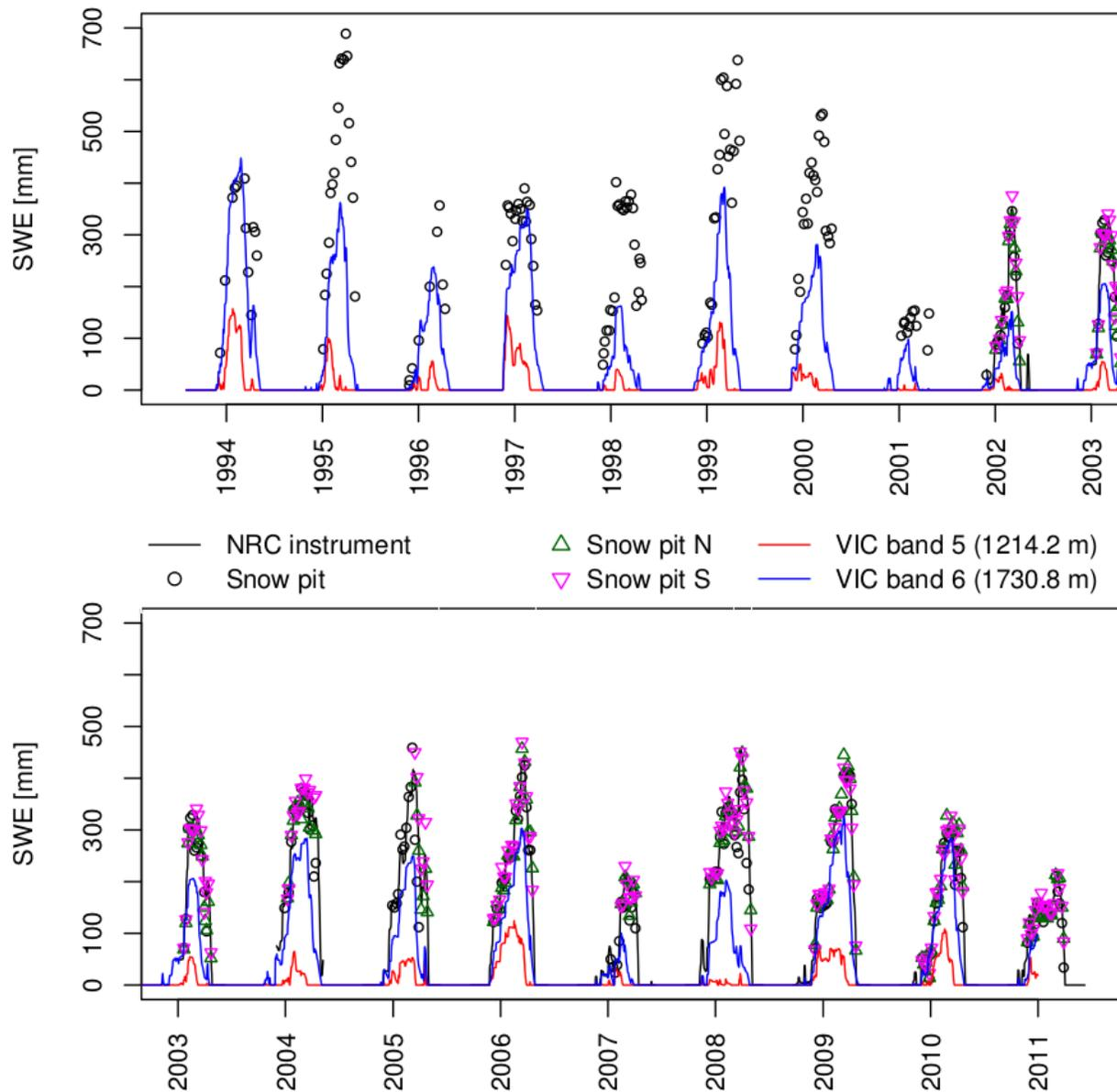
Fig 4: Snow water equivalent from the Col de Porte site. The NRC instrument series is drawn as a black line while the three manual snow pit measurements are shown as symbols. The station is located at 1325 m above sea level. The two nearest elevation bands are shown as lines; band 5 (at 1214.2 m, red line) and band 6 (at 1730.8 m, blue line).
